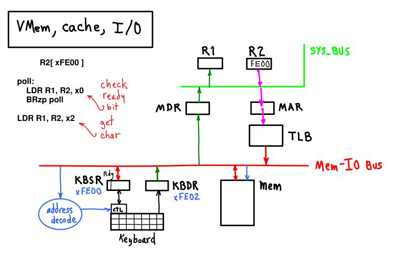
Device address decode recognizes xFE00 and xFE02. Keyboard data moved to R1.
