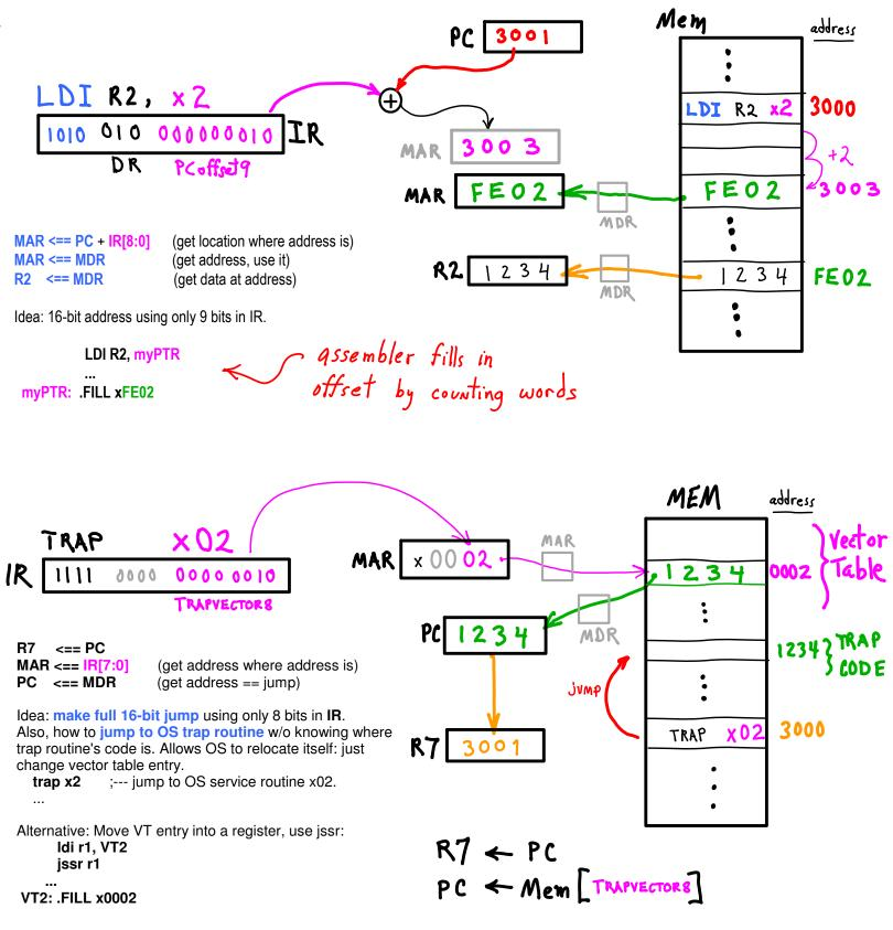
Aside: Using what we had above to eliminate ldi, we could eliminate both LDI and TRAP instructions from the LC3's ISA: we would have two unused opcodes to play with.
