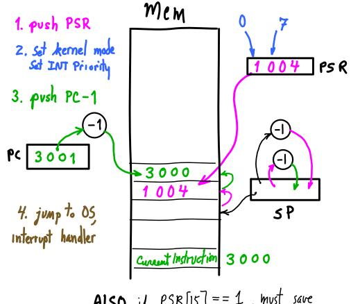
ALSO, if PSR[15] == 1, must save SP, and switch to SUPER'S STACK. See R6 save/restore handware near ALU.
