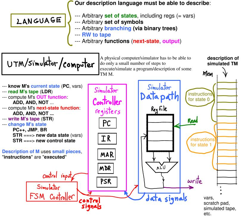
FSM Controller uses registers (e.g., PC) to remember:
