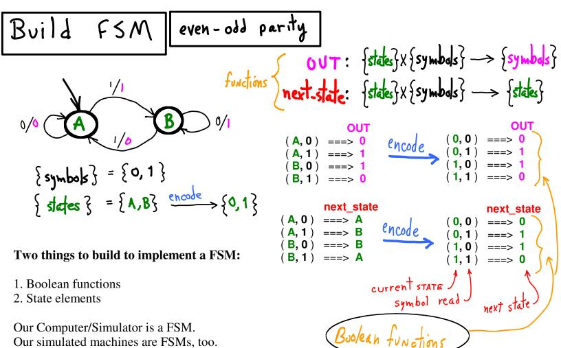
Our Computer/Simulator is a FSM. Our simulated machines are FSMs, too. Turing Complete/Universal (can simulate any TM) we need:
