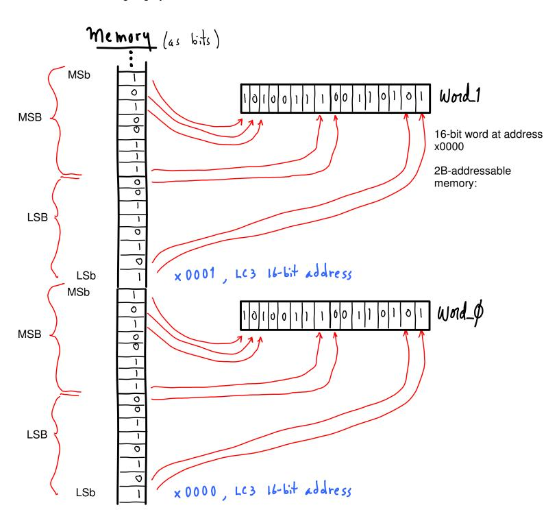
Suppose we extend LC3 addresses by one bit (17-bit addresses) to have a Byte-addressable memory:
