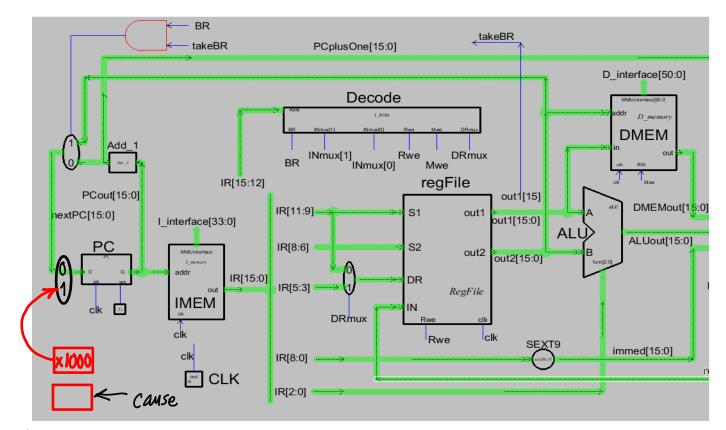
Add a MUX to PC Set MUX -> Jump to x 1000, dispatcher Why? "Cause" stored in Cause-negister, for interrupts function number in RØ, for syscalls. Add new instruction to access cause reg.
