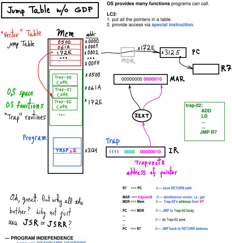
jump via STANDARD VECTORS --- OS convention (see OS manual) Write VT at boot time, functions are relocatable.
