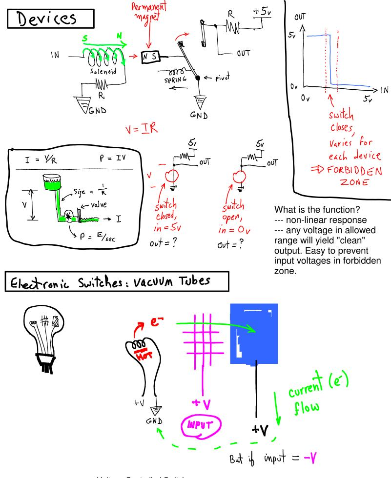
Voltage Controlled Switch faster, more reliable, less power
