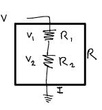
Resistors connected in SERIES.
