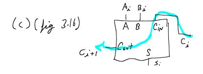
Each 1-bit adder requires 3 gate delays for the Ci signal to propagate to the Ci+1 output. For the first stage, getting C1 does not depend on C0 because C0 = 0 always, but C1 also depends on A1 and B1 which takes 3 delays. Since there are 4 1-bit adders chained together, Ci to Ci+1, the total delay is 4\*(3) = 12 delays.
