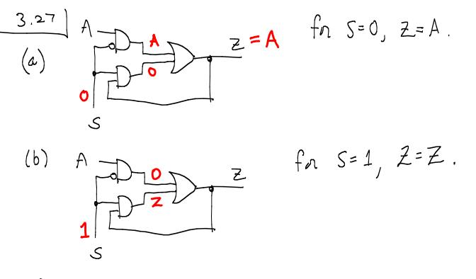
( $\zeta$ ) Yes, this is a latch. When S = 0, the latch is transparent with Z = A, whatever A is (0 or 1), Z simply follows A. But, when S = 1, The A input is ignored, and the output remains Z, whatever Z was before S changed to 1.
