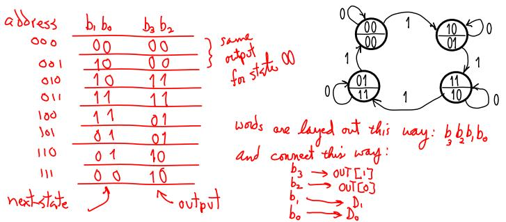
**Q.** How could the table above be recoded into a linear form suitable for simulation by a Universal Turing Machine? (Assume bit b<sub>0</sub> of M's output is used to implement moving its R/W head left or right, and bit b<sub>1</sub> is its output symbol. At the clock tick, the R/W head moves and state changes.)
