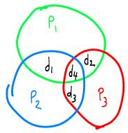
Code / Single Error Detection / Single Error Correction )
