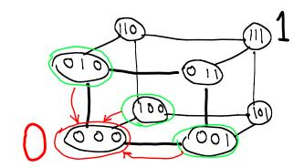
1-bit Correction, 2-bit Detection
