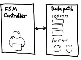
We like to separate state into two "types", control and data state. Eg., some state elements are for "control" state, and some are for "data" state.
