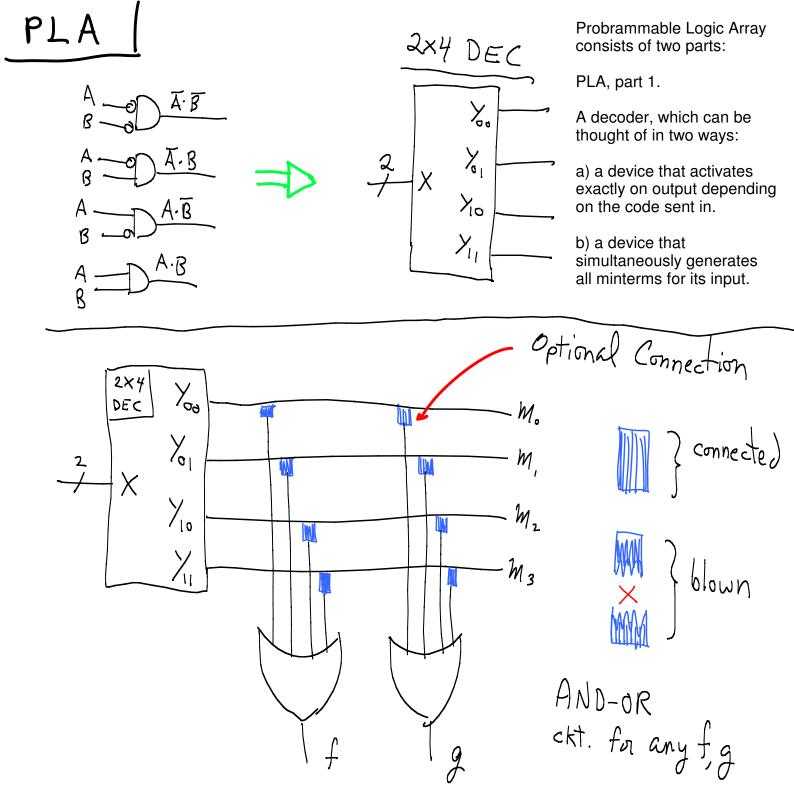
PLA, Part 2. A means of OR'ing minterms to produce function outputs.
