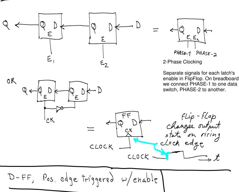
We often want to control whether or not the FF will be written into when the clock pulse arrives: add an "enable" input. When enable is 0, the current state is written back into the FF. Otherwise, D is written.
