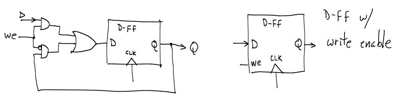
If there is no feedback path from Q to D, we do not need a flip-flop, we can use a write-enable latch instead. Datapaths sometimes can use latches.
