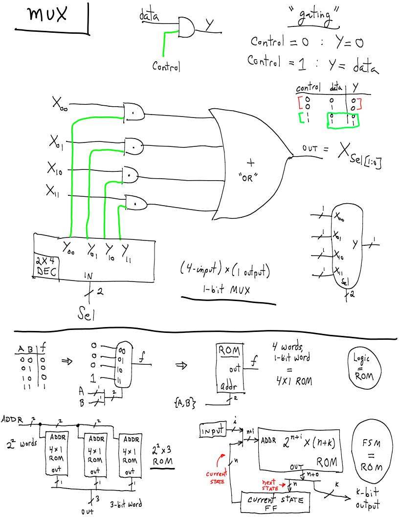
FSM in ROM ( n-bit state, i-bit input, k-bit FSM output )
