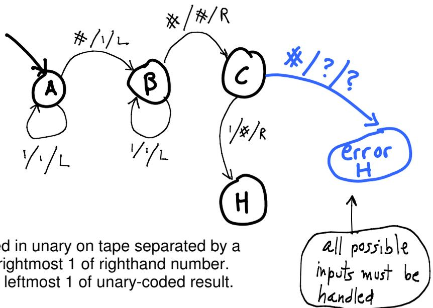
User Manual: Start with two numbers coded in unary on tape separated by a single blank, and RW-head positioned on rightmost 1 of righthand number. Machine halts with RW-head positioned at leftmost 1 of unary-coded result.
