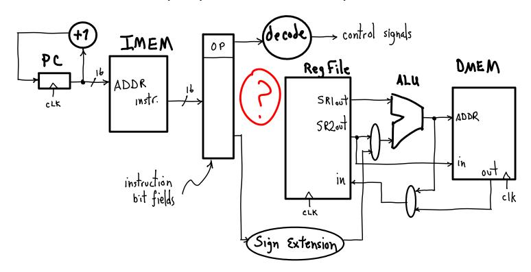
There are no select lines into RegFile to control what is fed to SR1out and SR2out: we need to have SR1 and SR2 inputs from the instruction bits. We also need DR input to select which register is written. There are two memories: IMEM and DMEM for instructions and data, respectively.
