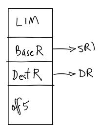
We have limited immediate values we can use. LIM gets us 5 bits, unsigned, loaded into the low bits of DestR. Using this with SHL (see below), will allow us to get 16 bits into a destination register using 4 LIM instructions with 3 SHL instructions. BaseR could be used as a shift left amount?
