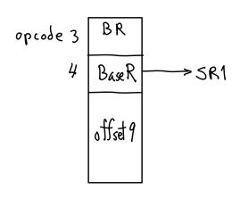
All instructions have bits instruction[15:13] as the opcode. Instruction[12:9] designate the Base Register for addressing. This allows for 16 registers, which would help us a lot. SR1 always selects the Base Register for address arithmetic in every instruction.
