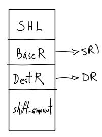
SHL shifts bits left in DR by the number in the "shift-amount" field. I don't know what BaseR would be used for. It could be used as the source so DestR could be a different register.
