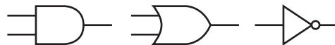
FIGURE C.2.1 Standard drawing for an AND gate, OR gate, and an inverter, shown from left to right. The signals to the left of each symbol are the inputs, while the output appears on the right. The AND and OR gates both have two inputs. Inverters have a single input.
