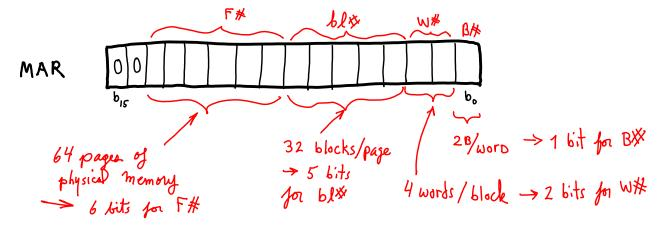
The same address bits can be thought of in this format: [ TAG, index, W#, B# ]:
