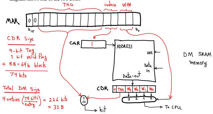
Q. Draw the wire connections from the MAR to the CAR, to the MUX select, and to the comparator. Indicate the total number of bits in the CDR and total DM bits.
