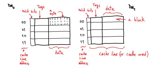
Note that each DM is a small memory, with an address port, a data-out port, a data-in port, and a write-enable, as shown below. We can think of this memory as having an address register equivalent to an MAR, the Cache Address Register (CAR), and an equivalent to the MDR, the Cache Data Register. The diagram shows one of the two DMs.
