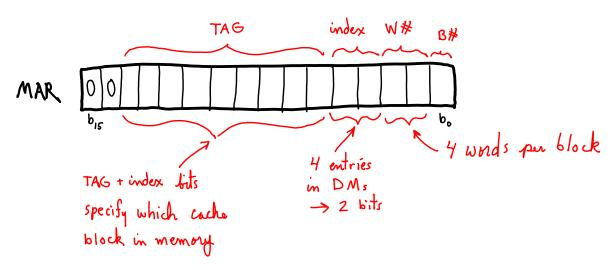
Q. The figure below shows the cache's two DMs. Indicate which blocks form each set and the index for each set.
