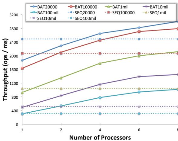
**Figure 5: Throughput of BATCHER and sequential skip list insertion for various initial sizes of skip lists (higher is better).**
