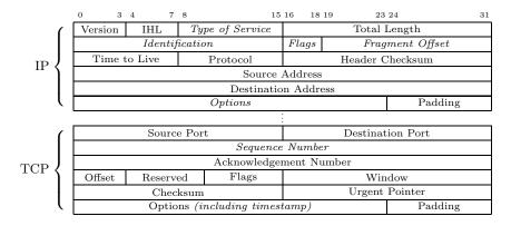
Fig. 1. Basic TCP/IP header structure
