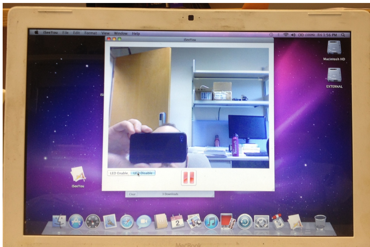
Figure 3: iSeeYou running on a white MacBook “Core 2 Duo” capturing video from the internal iSight with the LED (the black dot to the right of the square camera at the top, center of the display bezel) unilluminated.
